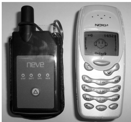
Figure 2: The Neve GPS device in comparison to a standard Nokia mobile phone
